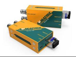
The FE1121 3G-SDI Fiber Optic Extender is a transmitter/receiver kit supporting single-mode LC simplex fiber extensions up to 20km. It is a miniature-style extension solution that supports all SDI formats resolution up to 1080p with audio and metadata, also supports level A and level B. It features a local SDI loop out and dual SDI outputs and supports 3G/HD/SD SDI signals.
